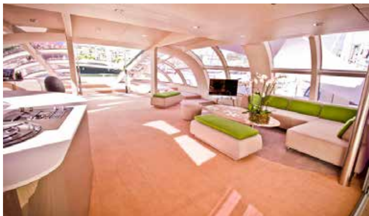
The integrated variable transparency glass lightens or darkens according to the amount of sunlight.
