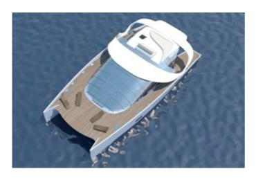
Power will come from twin 260hp diesels driving water-jets, which will push this big cat up to an intentionally modest top speed of 20 knots to keep fuel consumption and emissions down.
